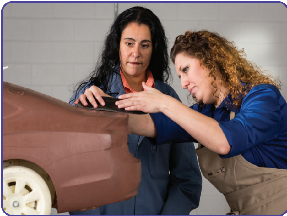
The design team might have a clay sculptor who models the vehicle out of clay.
