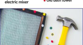
▲ 1. Thumbtack a mesh screen tightly across a frame (it could be an old picture frame). Use a hammer if necessary.
