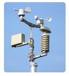
An **anemometer** measures wind speed.
