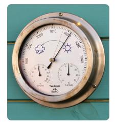
A **barometer** measures changes in air pressure.
