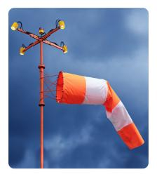
A **windsock** or **weathervane** measures wind direction.
